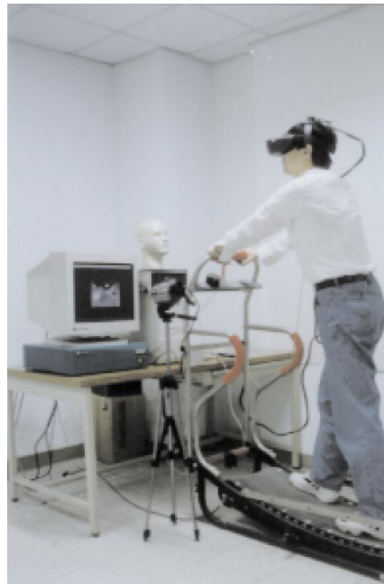
Fig. 6. The SpaceWalker system for a building walkthrough
